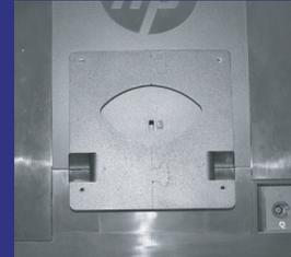
The MAK-HPCP4300 is a custom mount adapter bracket designed specifically for the HP Compaq Pro 4300 AiO Business PC. The stand is first removed from the 4300, then the mount adapter is attached to the back of the computer using the same holes and hardware. When installed, the 4300 AiO is ready to be attached to a VESA 100 compliant mounting device providing the correct weight capacity.
